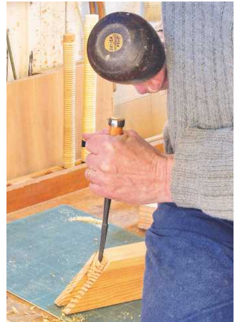
▲ Pic.5 Chopping the slot for the tenon
